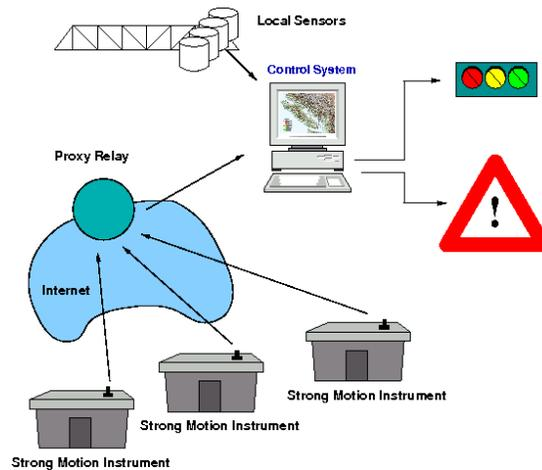
Figure 4. A regional network supporting an on-site traffic control system.
